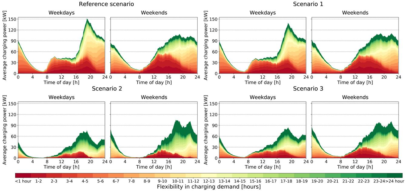
Fig. 2: Average charging power and average flexibility in EV charging demand on weekdays and weekend days in the studied LV grid for the four scenarios introduced in section IV-A.
